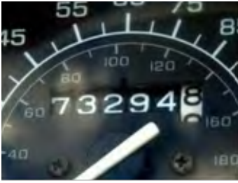
Wheel tick provides information about distance traveled
