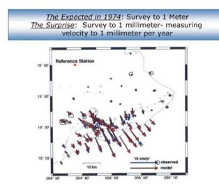
Figure 7. Continuous observation of earth crustal motion with a precision of better than a millimeter: distributed slip on Kilauea volcano, Hawaii. **Summary.** Many technologies came together to make GPS operational, none more revolutionary than the signal structure demonstrated by 621B at White Sands, and selected by Parkinson during the Lonely Halls meeting. Virtually all high-precision uses of GPS depend on the characteristics of this signal.
