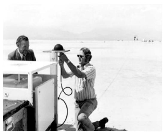
Al Gillogly, Aerospace engineer (left), setting up the critical tests of prototype GPS receivers at WSMR in 1970.
