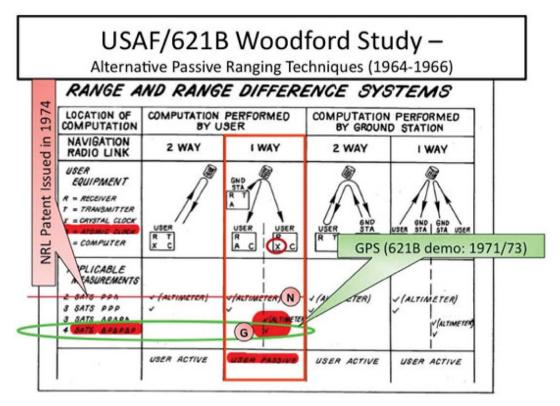
Figure 5. Summary of the alternative satellite-based navigation techniques from the 1964–66 USAF/621B study. The most capable option, circled in green, became the basis for the White Sands prototyping and testing, and then evolved into GPS. NRL applied for a patent on the less capable technique (red line) four years after the Woodford/Nakamura Study was completed.
