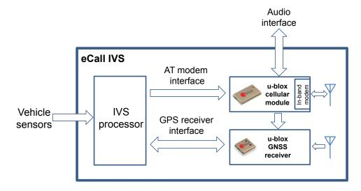
Fig. 6: The u-blox IVS eCall system
