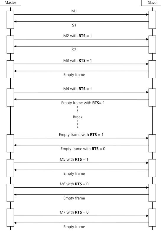
Figure 20: Flow control – both sides signaling
