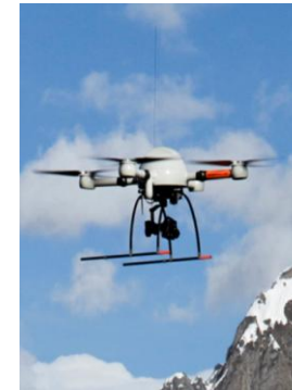
Microdrone md4-1000, using u-blox positioning products for navigation and control
