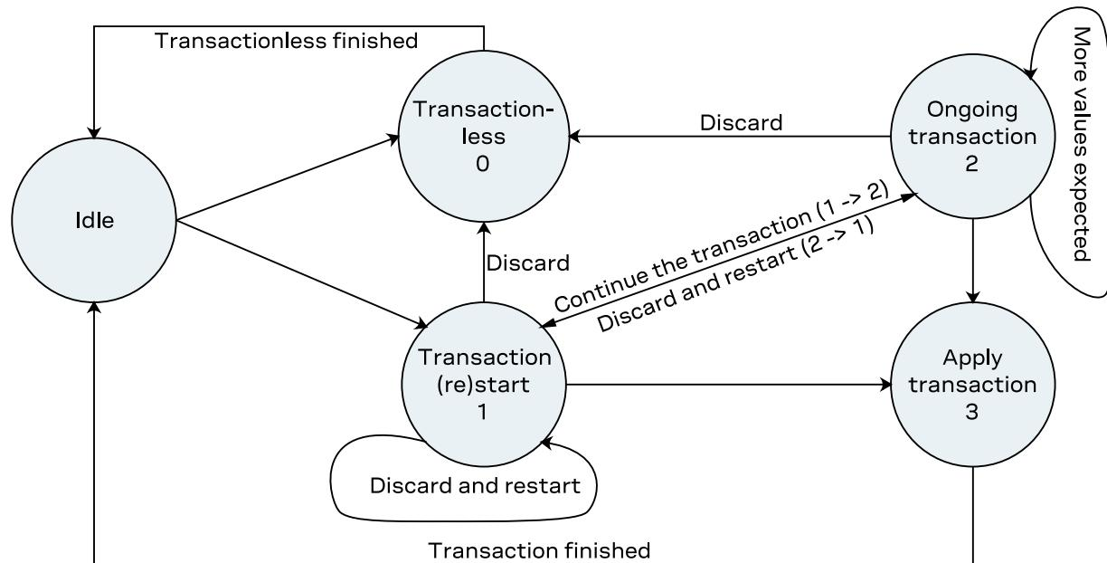
When starting a transaction, specify the layer(s) to apply the changes to. This list of configuration layer(s) must be observed throughout the transaction states. Modifying the configuration layer(s) mid-transaction causes the transaction to be aborted and consequently, no queued changes will be applied.
