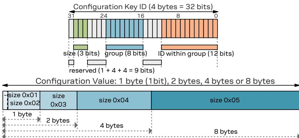
A configuration key ID is a 32-bit integer value, which is split into the following parts:
