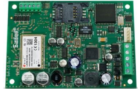
Satel, Poland Wireless security module with u-blox' GSM module
