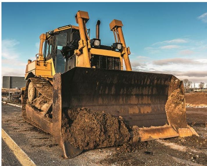
Figure 6: Heavy machinery control – blade leveling and heading, base and rover on the vehicle
