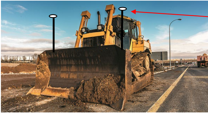
Figure 15: Antenna placement in heavy machinery/machine control application
