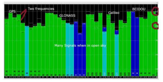
Figure 8: u-center Satellite Level view
