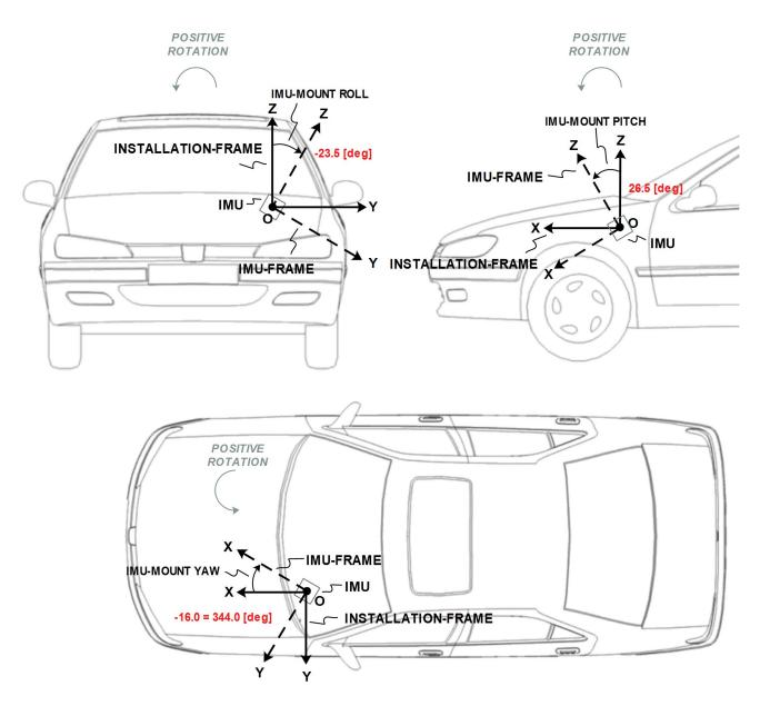
Figure 6: IMU frame and installation frame
