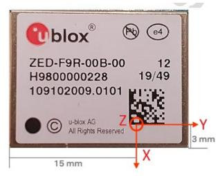
Figure 7: Orientation information. Z-axis points upwards.
