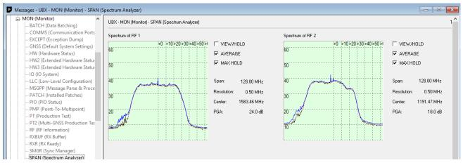
Figure 20: u-center UBX-MON-SPAN showing the spectrum at the L1 and L2 bands
