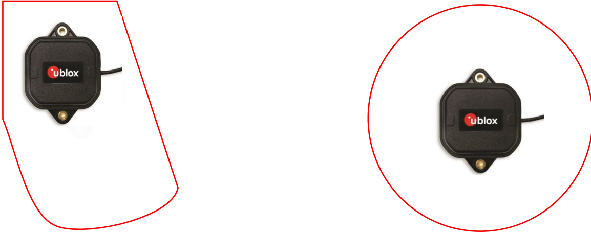
Figure 12: Non-uniform ground plane shape will offset the phase center (image on the left). Uniform circular ground plane (10 cm) provides best accuracy and performance (image on the right).
