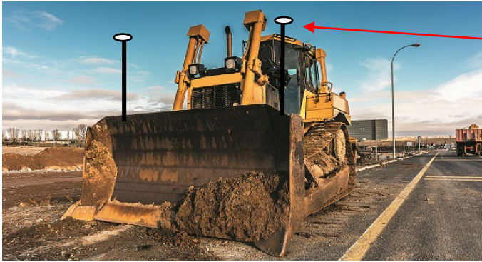
Figure 15: Antenna placement in heavy machinery/machine control application
