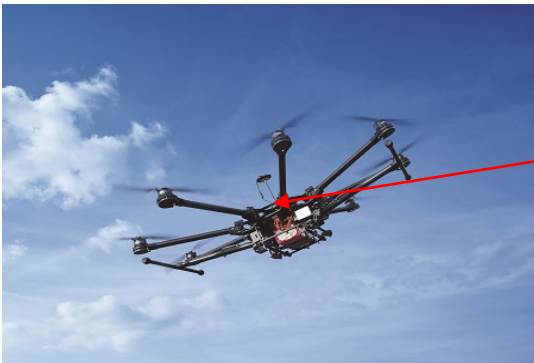
Figure 13: Drone application and recommended position of the GNSS antennas
