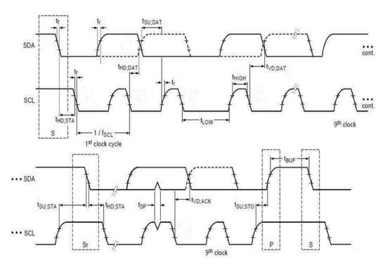
Figure 5: ZED-F9P-02B I2C peripheral specification
