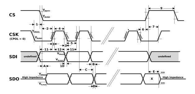
Figure 4: ZED-F9P-02B SPI specification mode 1: CPHA=0 SCK = 5.33 MHz
