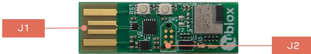
Figure 3: Available connectors, pinout, and designators
