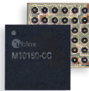
Small CSP33 package 2.39 x 2.39 x 0.55 mm
