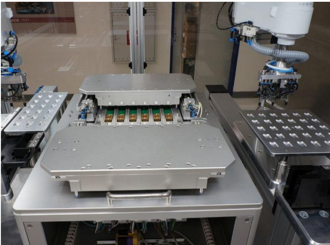
Figure 18: Automatic test equipment for module test
