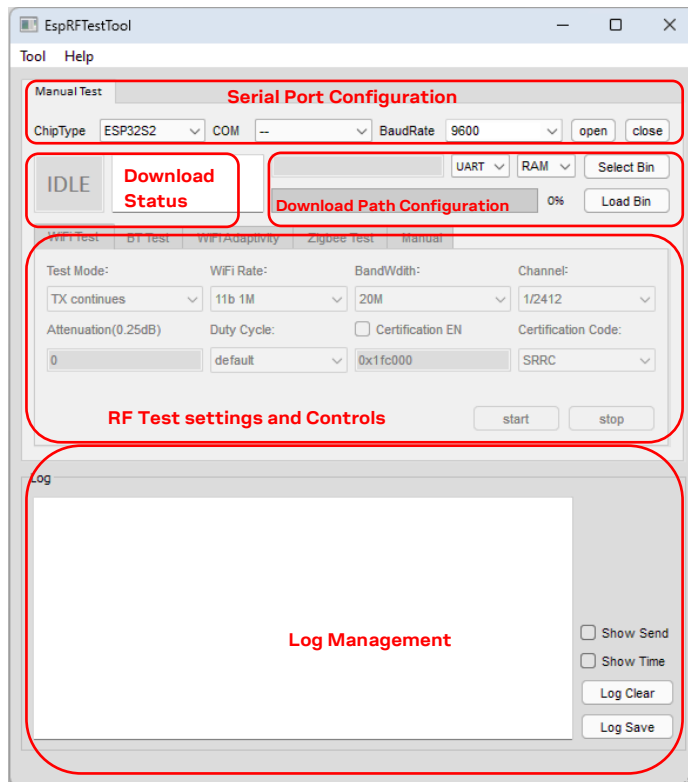
Figure 19: ESP RF performance test tool
