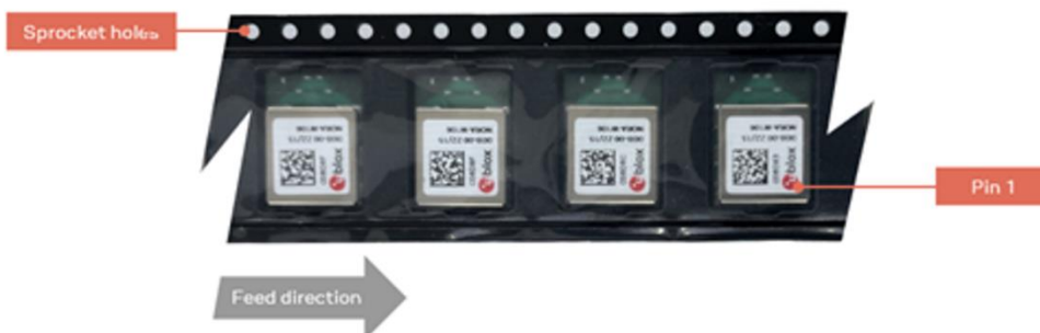
Figure 8: NORA-W406 module on tape orientation
