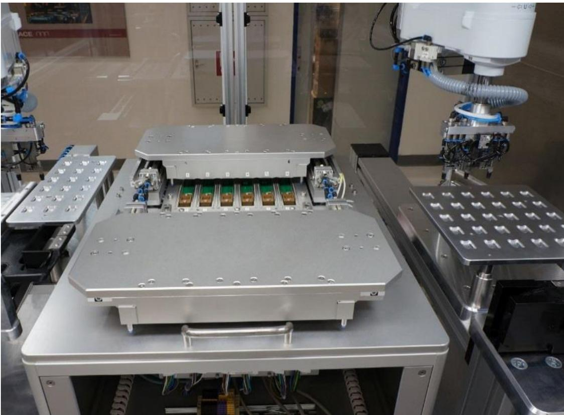
Figure 15: Automatic test equipment for module test
