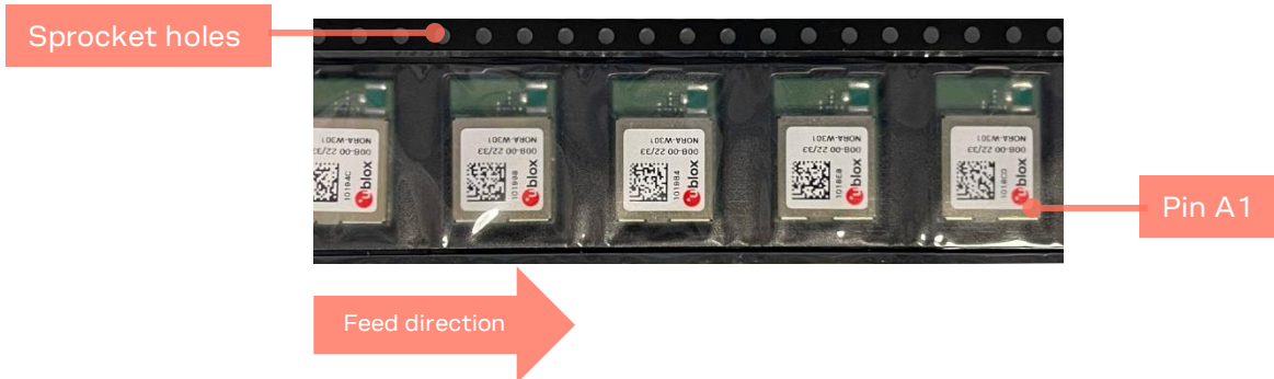
Figure 6: NORA-W301 module on tape orientation
