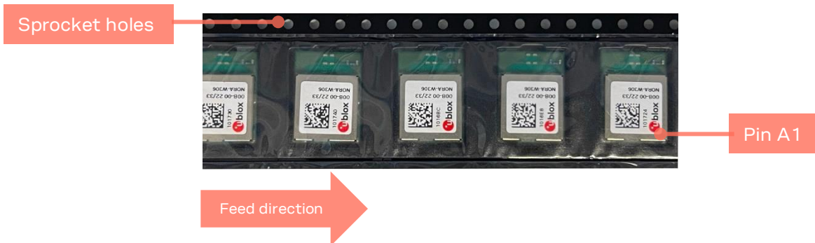
Figure 7: NORA-W306 module on tape orientation
