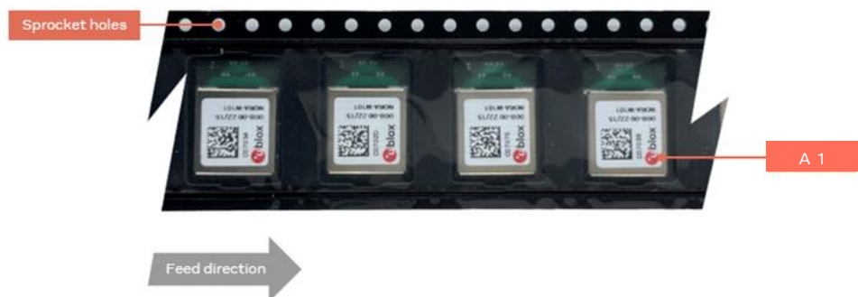
Figure 9: Orientation of NORA-B2 x6 module on tape
