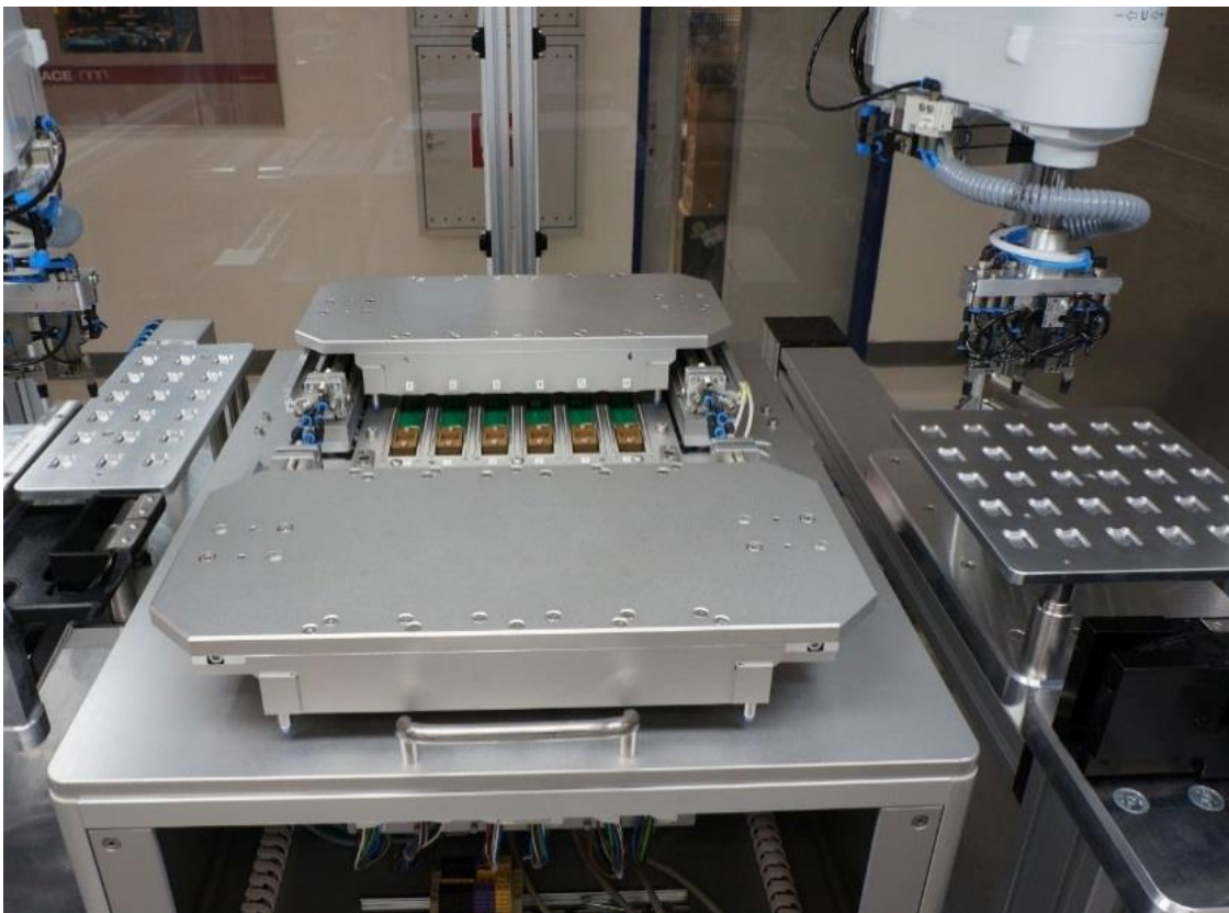
Figure 24: Automatic test equipment for module test
