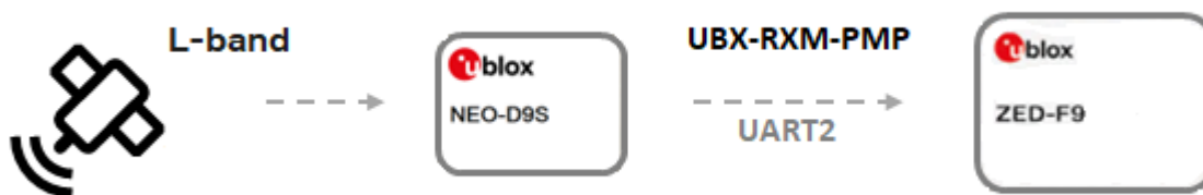
Figure 2: NEO-D9S and ZED-F9 connection
