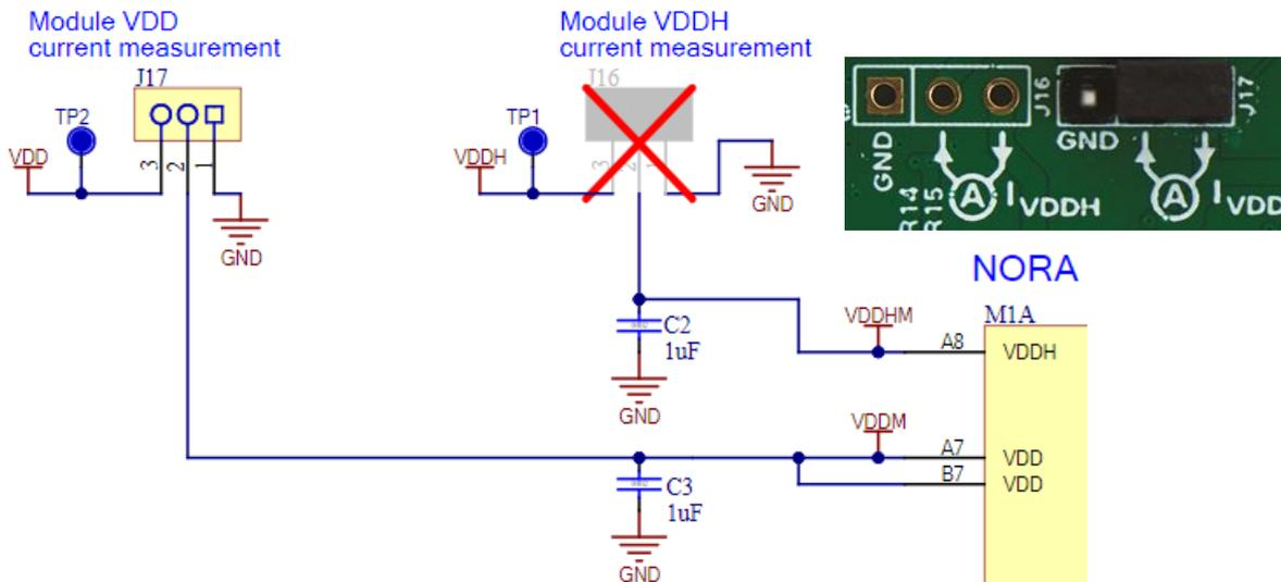
Figure 10: MINI-NORA-B12 current measurement
