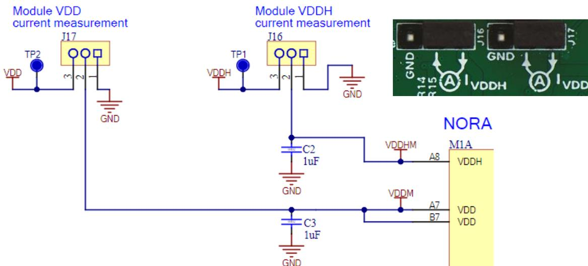
Figure 9: MINI-NORA-B10 current measurement
