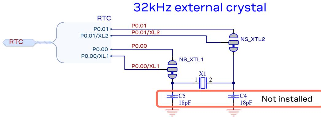
Figure 5: Schematic – 32 kHz crystal
