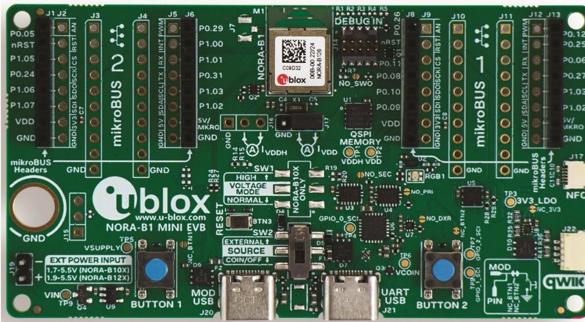
Figure 1: MINI-NORA-B1 rev C evaluation board (top view)
