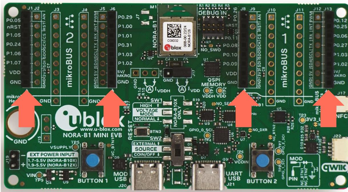
Figure 11: mikroBUS header location (header color may vary)
