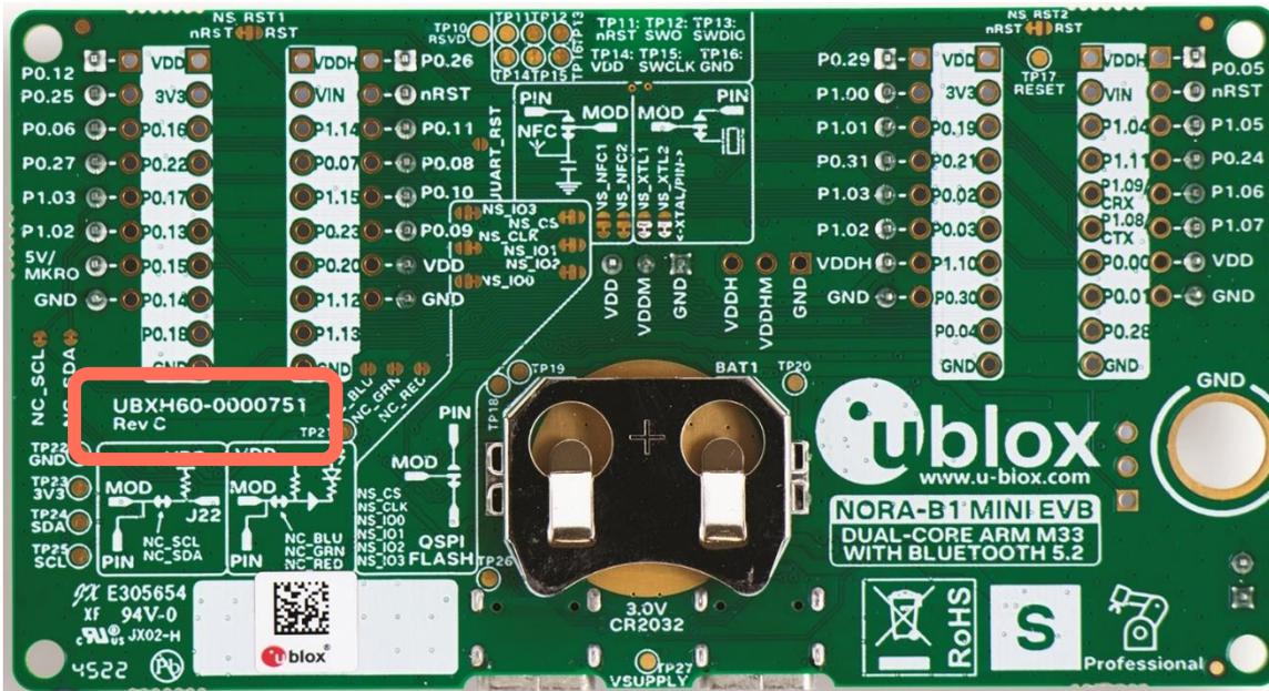
Figure 2: MINI-NORA-B1 rev C evaluation board (bottom view)
