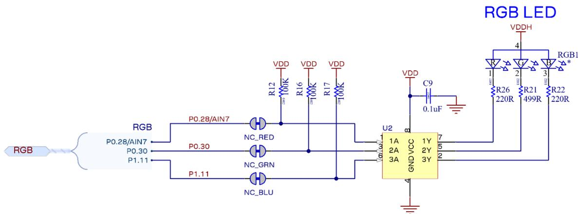
**Figure 4: RGB LED schematic**
