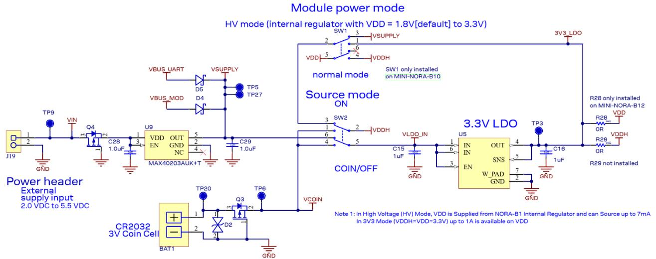
**Figure 3: MINI-NORA-B1 power schematic**
