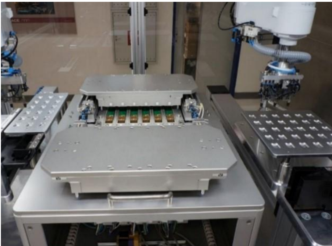
Figure 20: Automatic test equipment for module test
