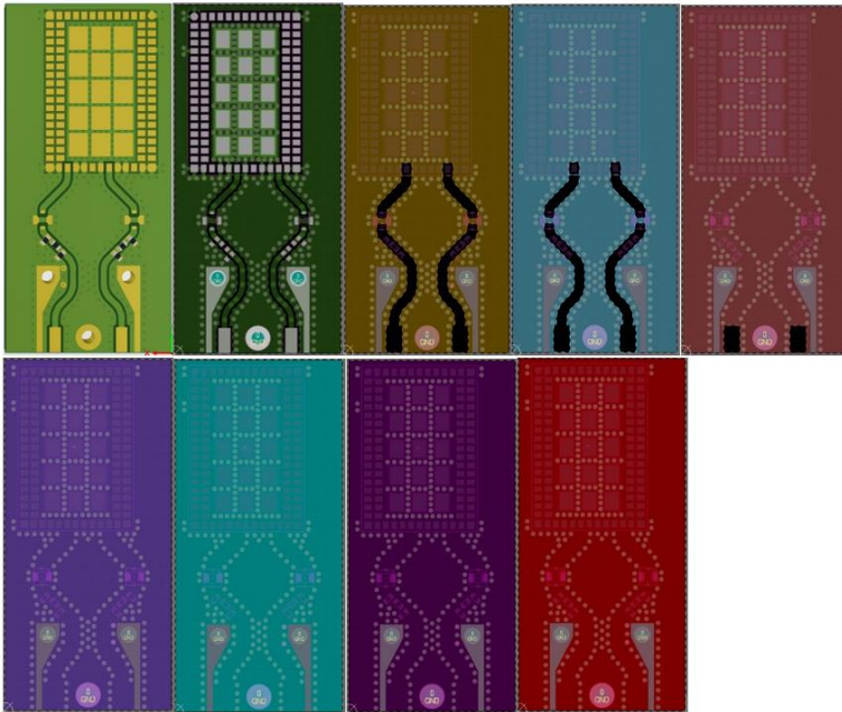
Figure 10: RF trace and ground design example
