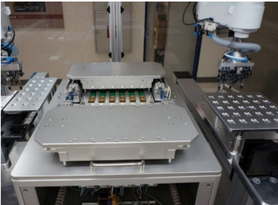
Figure 21: Automatic test equipment for module test
