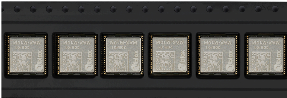
Figure 5: Orientation of the components on the tape
