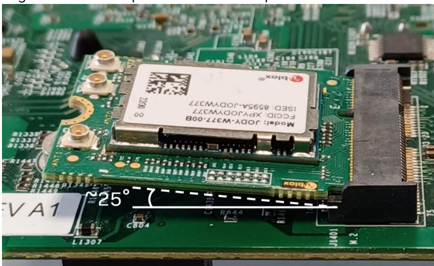
Figure 2: Inserting the M.2 card into the socket on the host computer board
