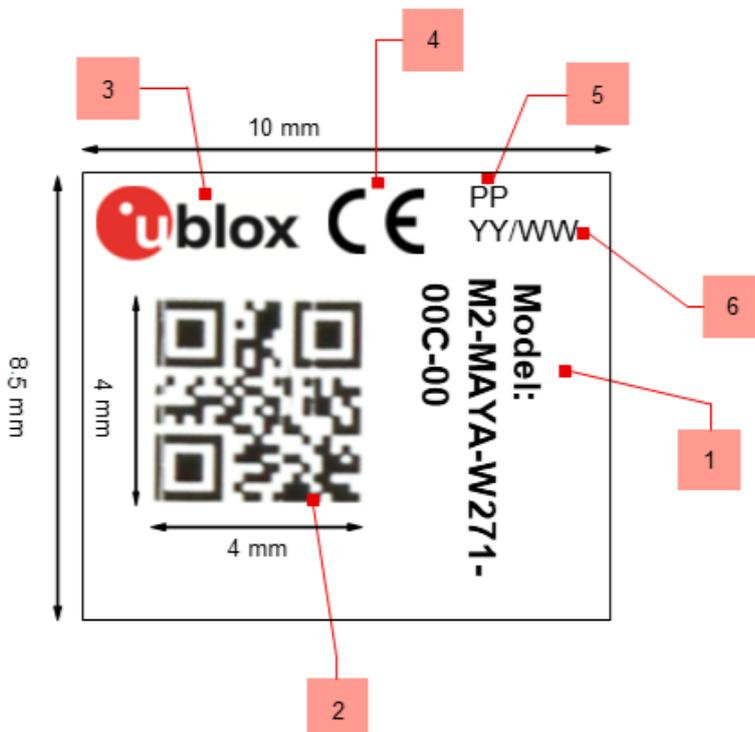
**Figure 12: Product label format with dimensions for M2-MAYA-W271**
