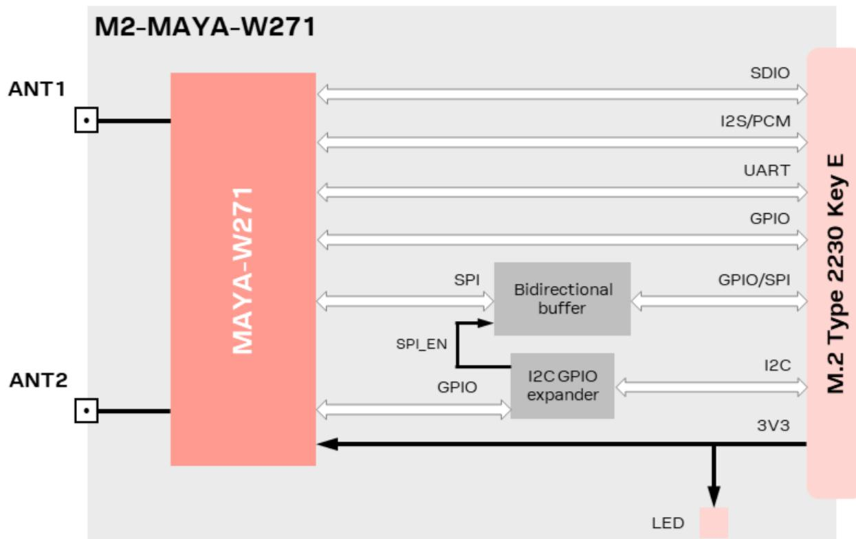
Figure 1: Block diagram of the M2-MAYA-W271 card
