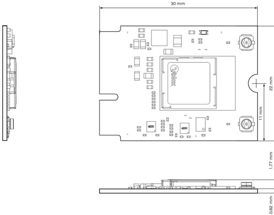
Figure 11: Physical dimensions of the M2-MAYA-W2 card
