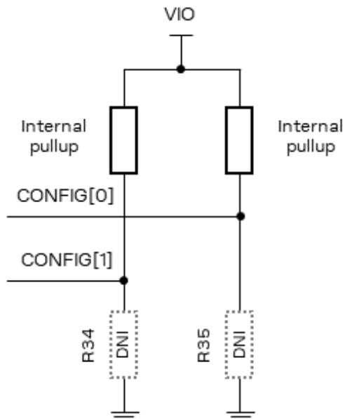
**Figure 2: Default configuration of the M2-MAYA-W2 boot pins**
