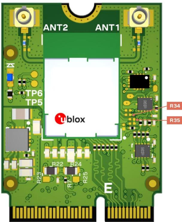
Figure 3: Position of resistors R34 and R35 on M2-MAYA-W1
