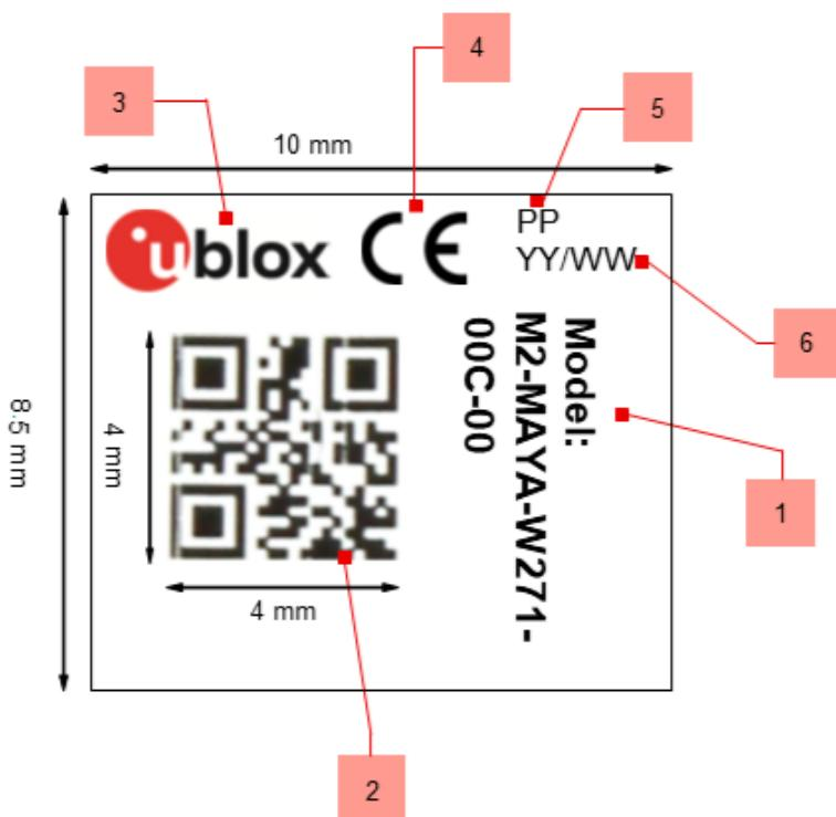
**Figure 12: Product label format with dimensions for M2-MAYA-W271**
