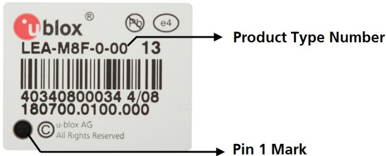
Figure 6: Location of product type number on LEA-M8F module label
