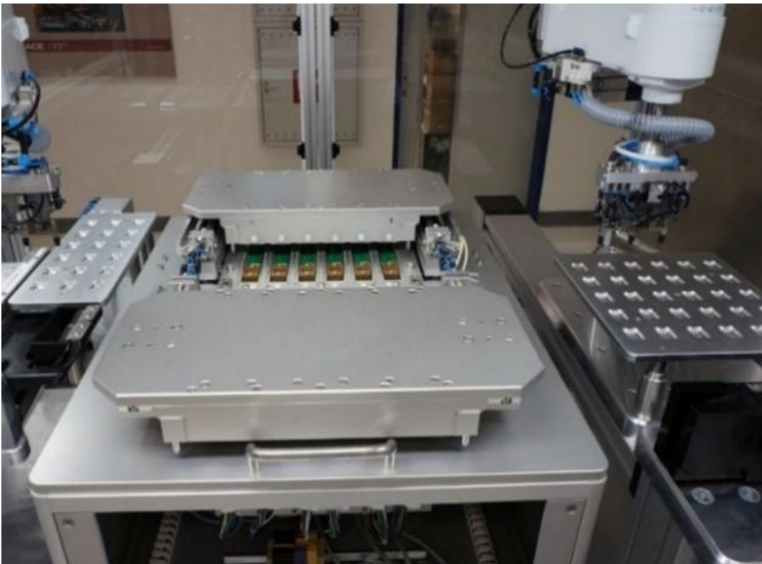
Figure 18: Automatic test equipment for module test
