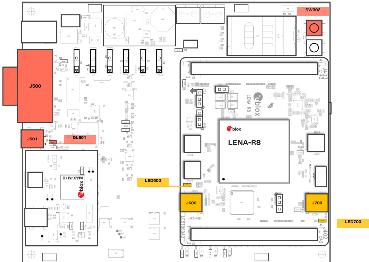
Figure 4: Set up local connectivity via USB or UART
