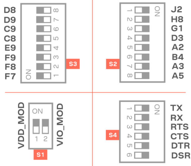
Figure 13: DIP switches on EVK NORA-W40
