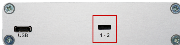
Figure 15: LNA control switch on the back panel
