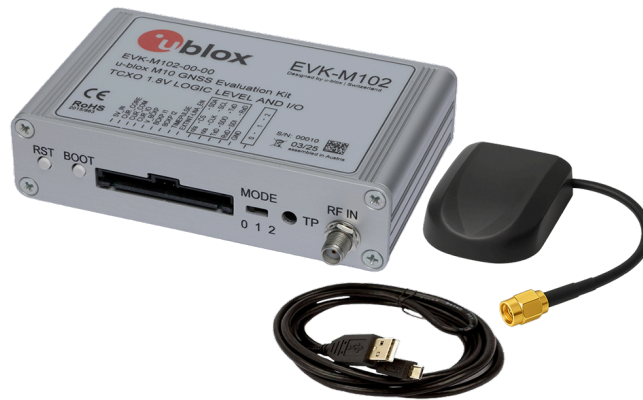
Figure 2: EVK, GNSS antenna, and USB cable included in the kit
