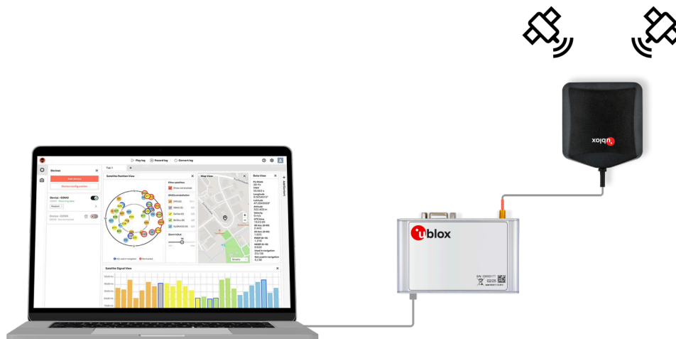
Figure 3: Connecting the EVK for communication
