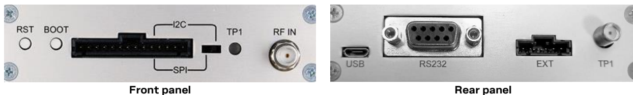
Figure 2: EVK-F9T evaluation unit – front and rear panels
