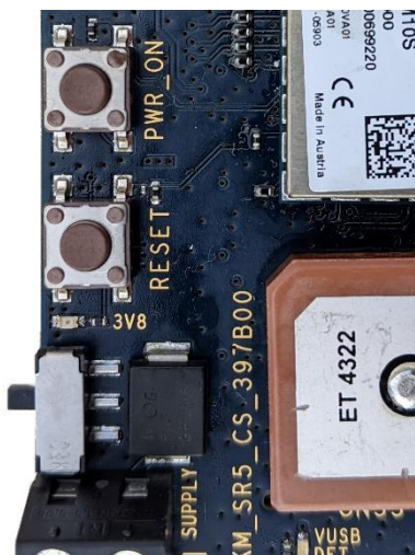
Figure 5: PCB detail showing the PWR_ON and RESET pushbuttons.
