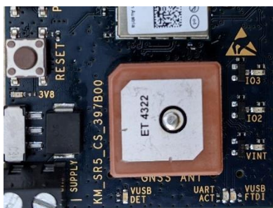
Figure 4: PCB detail showing the LEDs on the top side.
