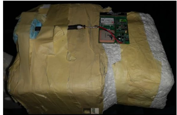
The voltage biasing has been done through the RF Cable of the anechoic chamber
