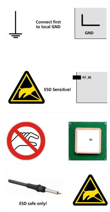
Failure to observe these precautions can result in severe damage to the GNSS receiver!
