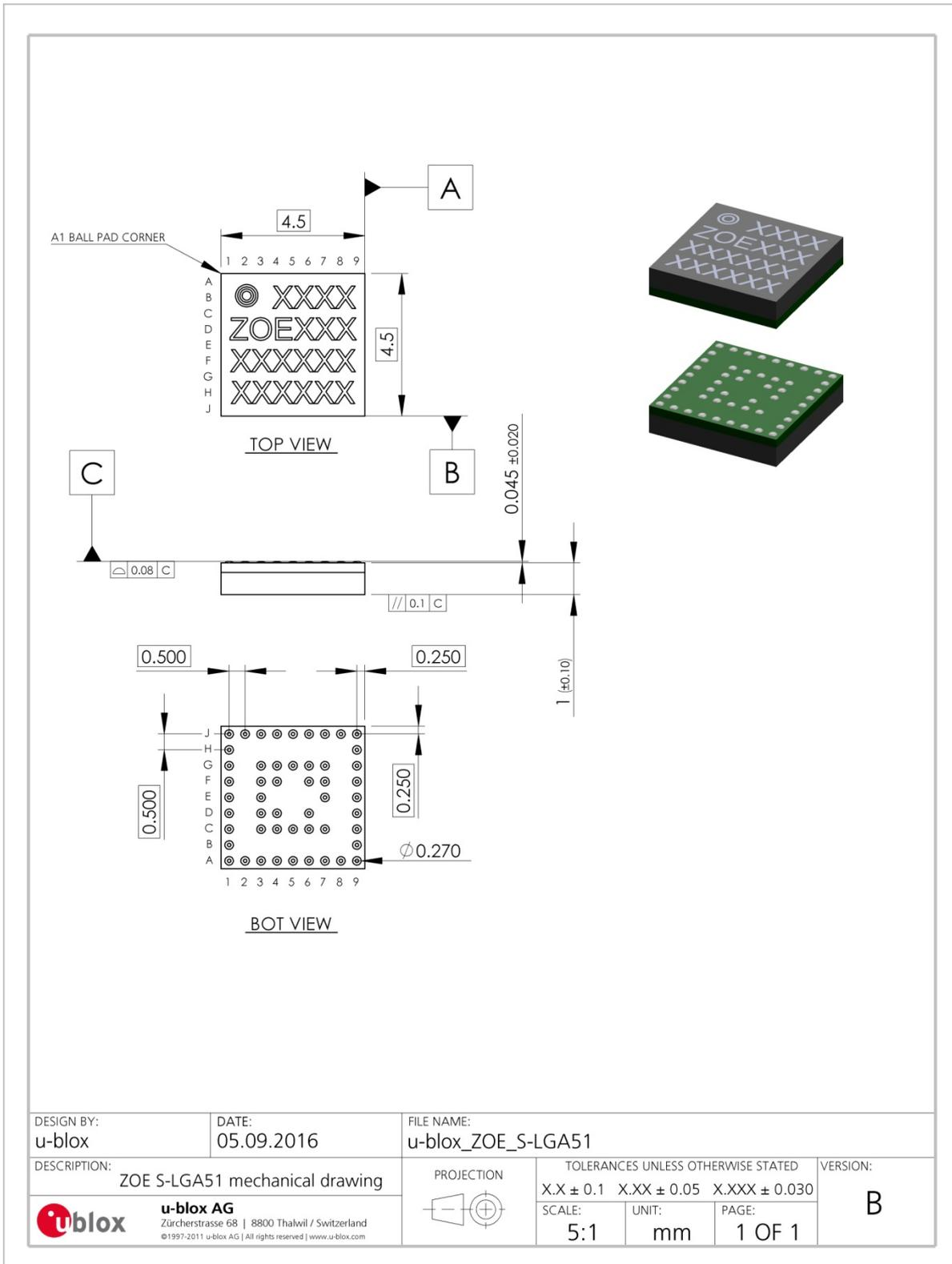
Figure 4: Mechanical drawing for ZOE-M8B (S-LGA), bottom view
