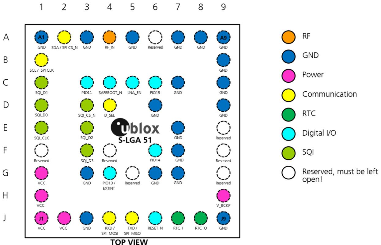
Figure 2: Pin assignment of ZOE-M8B (S-LGA51), top view
