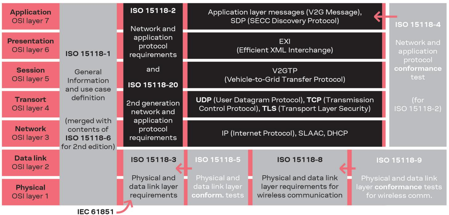
The components of the ISO 15118 standard, adapted from V2G Clarity
