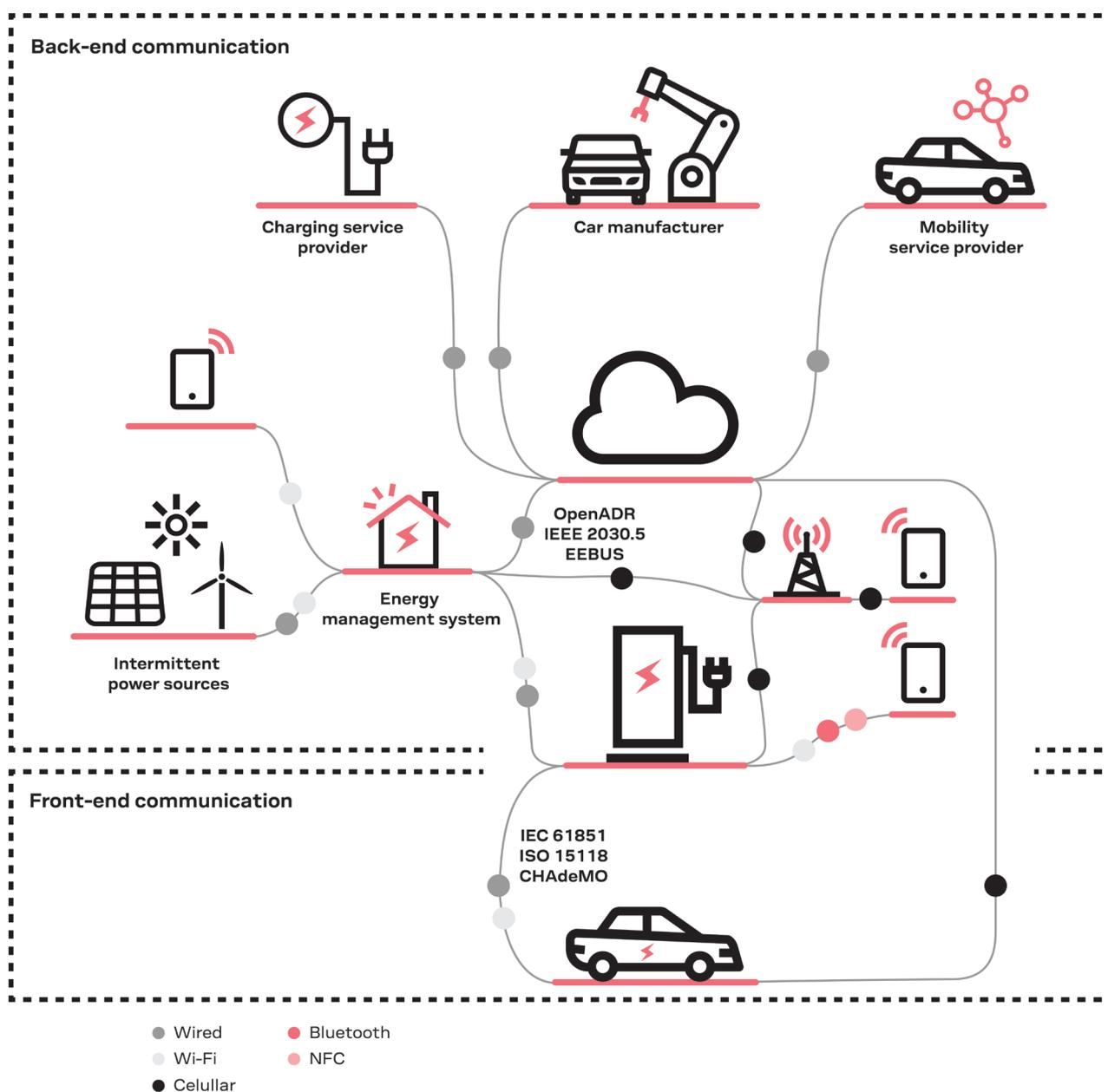
Front-end and back-end communication channels commonly used by EV charging stations.
