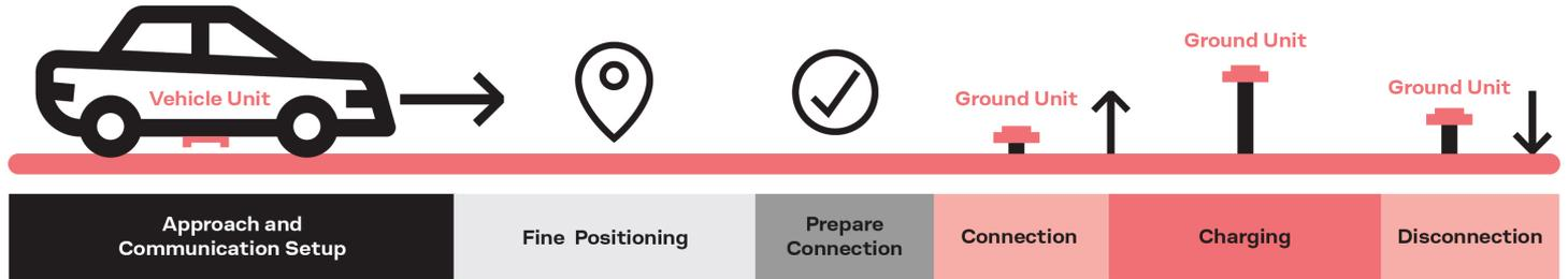
The sequence of events involved in wireless EV charging, which requires a wireless communication channel between the charging station and the vehicle.
