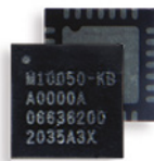
Small QFN28 package 4.0 x 4.0 x 0.55 mm
