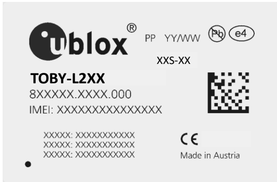
Figure 7: Example of TOBY-L2 series module label
