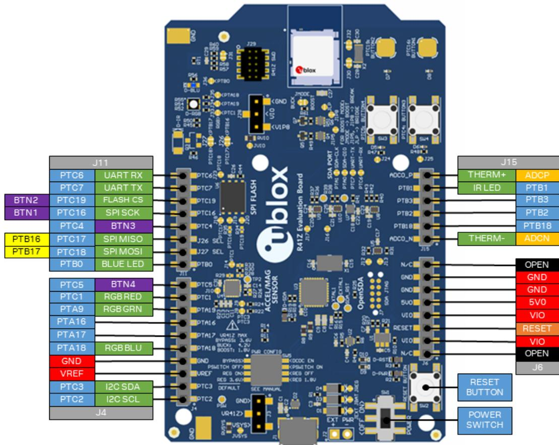
Figure 9: Expansion header pinout
