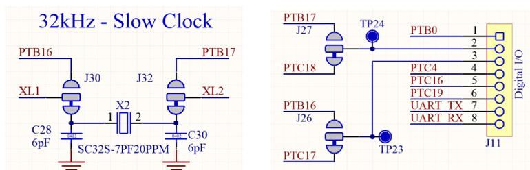
**Figure 16: Schematic: 32 kHz oscillator**
