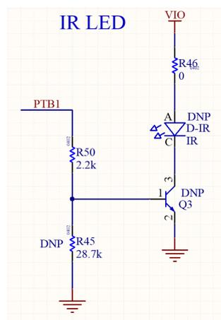
Figure 10: Schematic: IR LED
