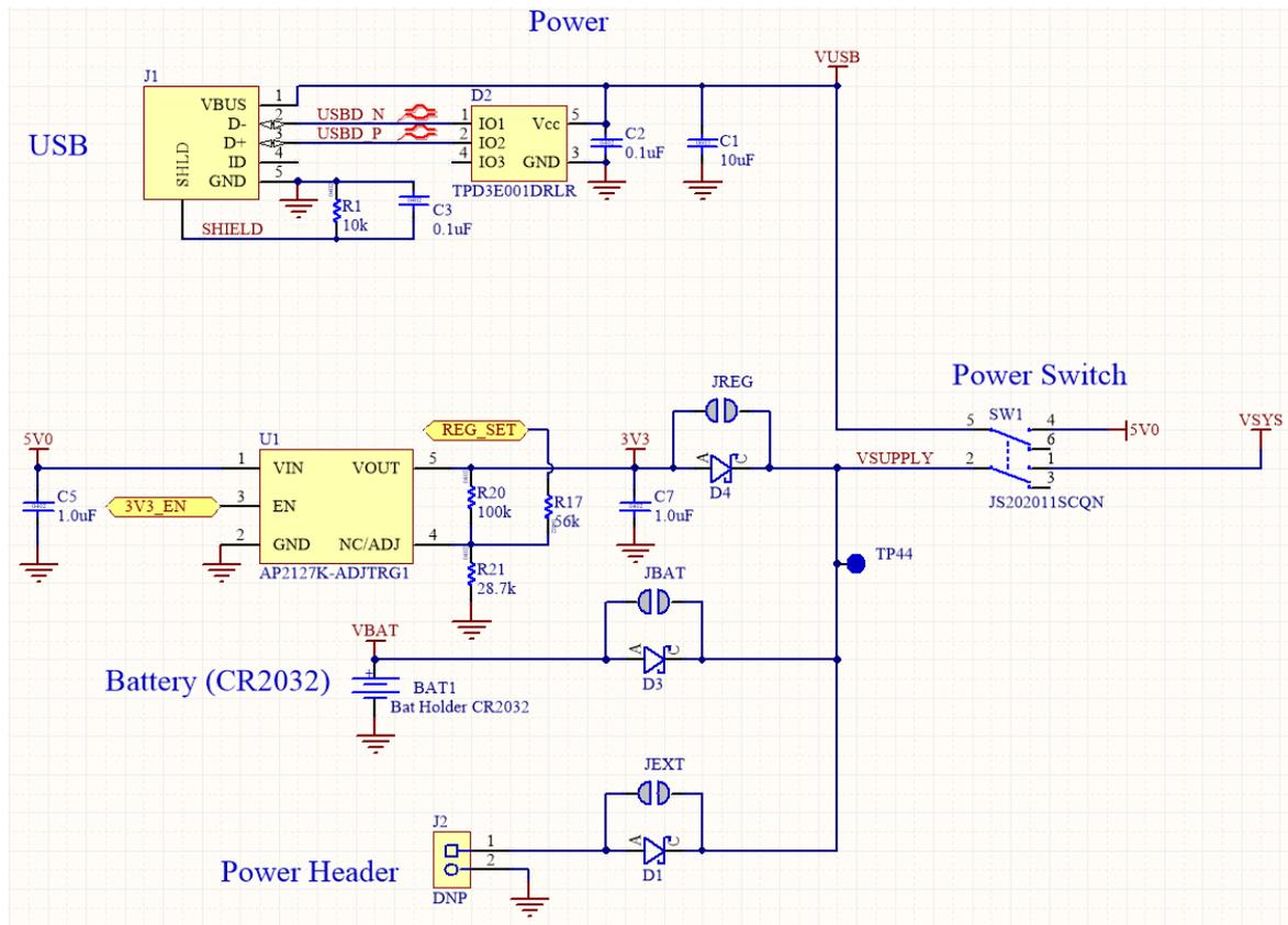
Figure 3: Schematic: Power supply
