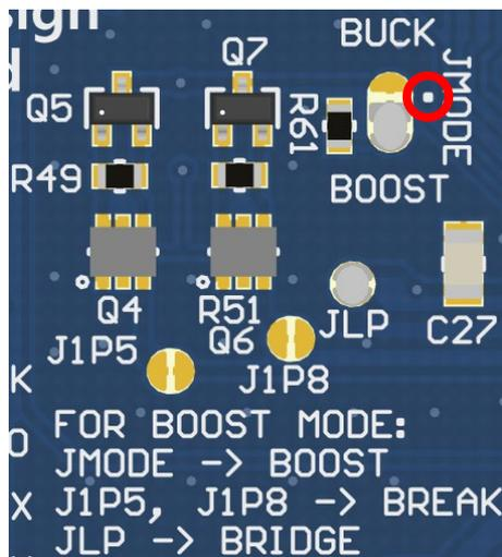
**Figure 6: Power configuration jumpers (Boost mode)**
