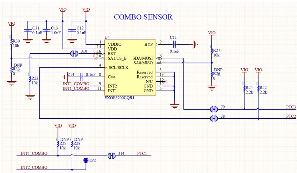
**Figure 15: Schematic: I2C combo sensor**
