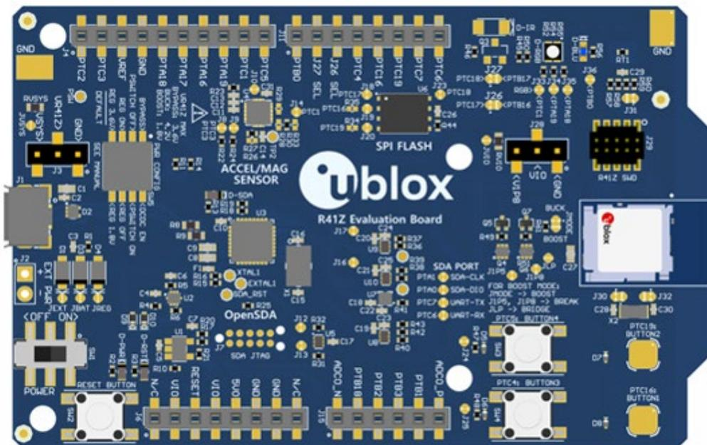
Figure 1: EVK-R41Z evaluation board (Top view)
