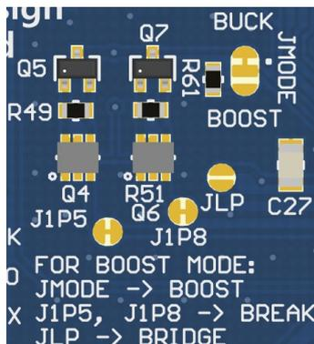
Figure 5: Power configuration jumpers (Default)
