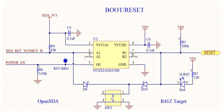
Figure 8: Schematic: Reset button
