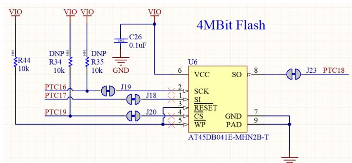
Figure 14: Schematic: SPI flash
