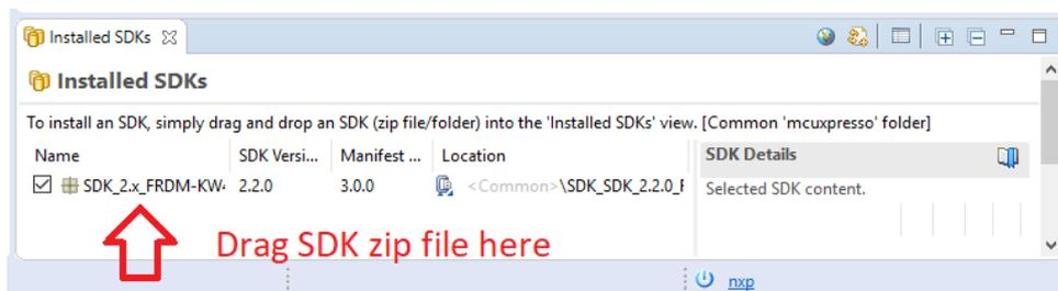
Figure 17: SDK installation
