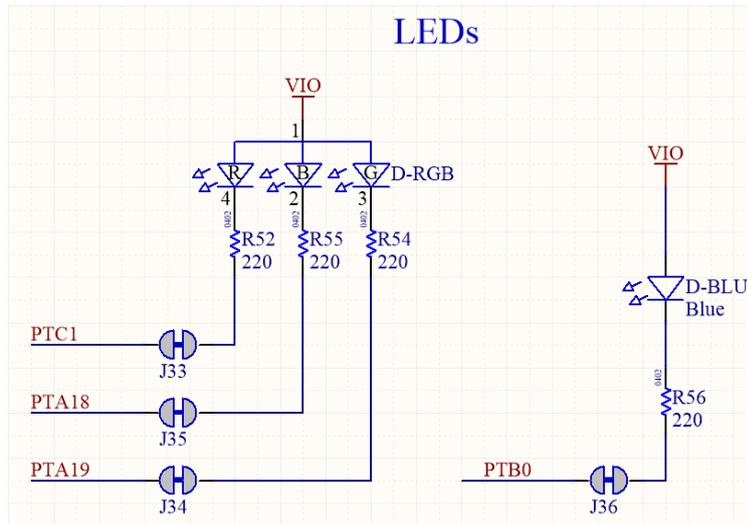
Figure 11: Schematic: User LEDs
