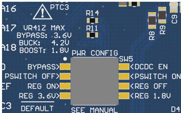
Figure 4: Power configuration switch
