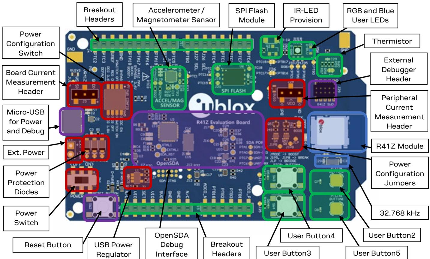
Figure 2: Evaluation board layout
