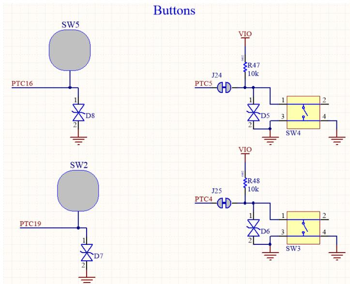
Figure 13: Schematic: User buttons
