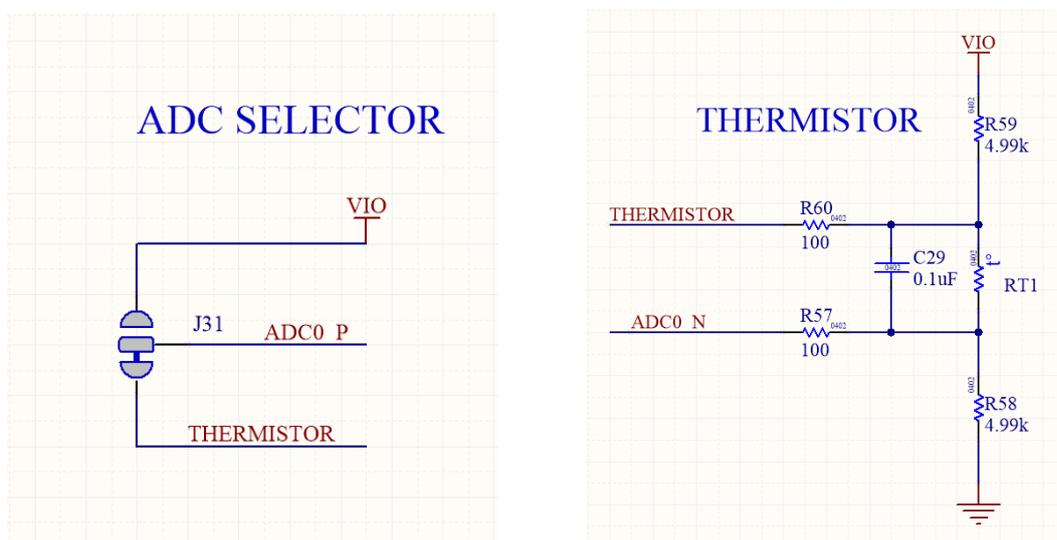
Figure 12: Schematic: Thermistor and ADC mode selection
