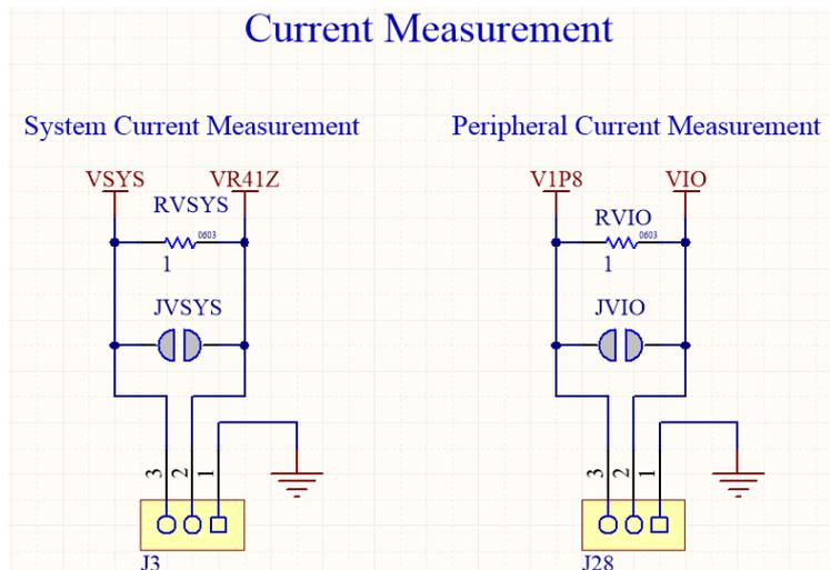
Figure 7: Schematic: Current measurement headers
