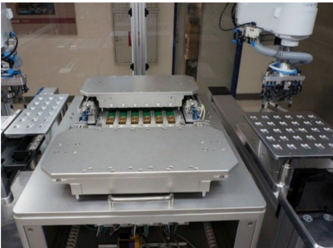
Figure 29: Automatic test equipment for module testing
