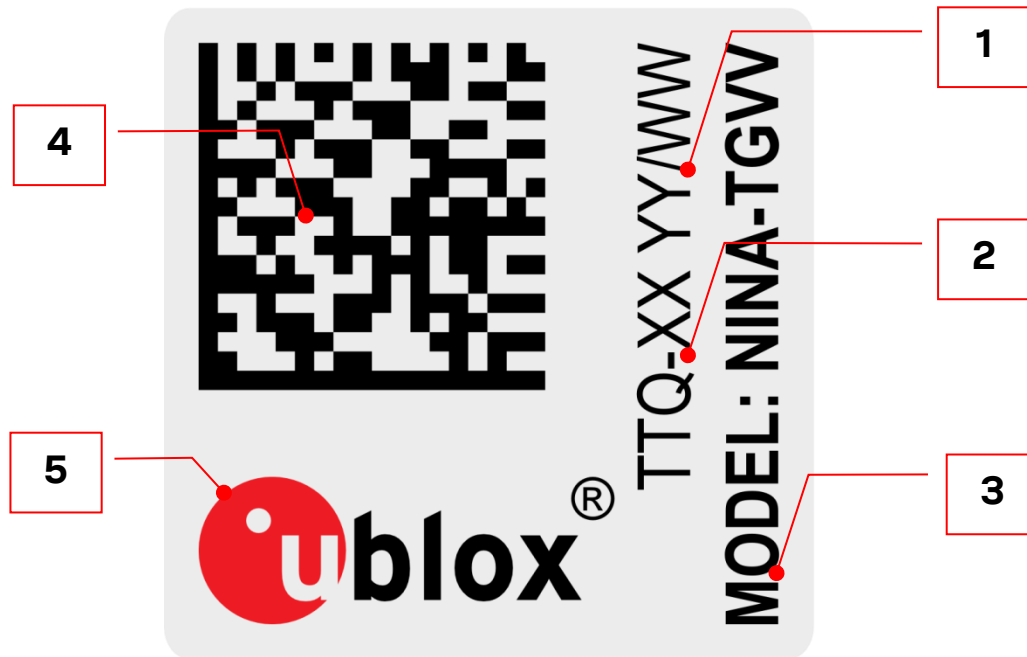
Figure 17: Location of product type number on the NINA-W15_DataSheet_UBX-18006647 module label
