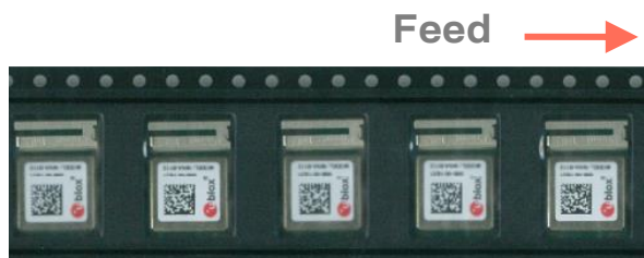
Figure 14: Orientation of NINA-W152/NINA-W156 module on tape
