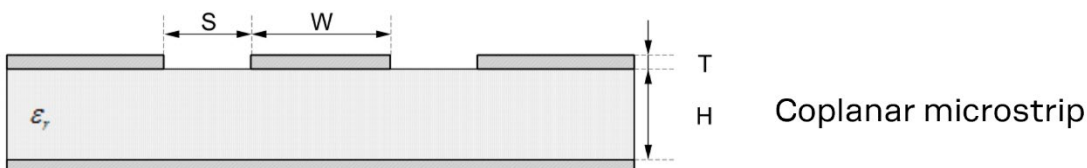
Figure 30: Coplanar microstrip dimension specification
