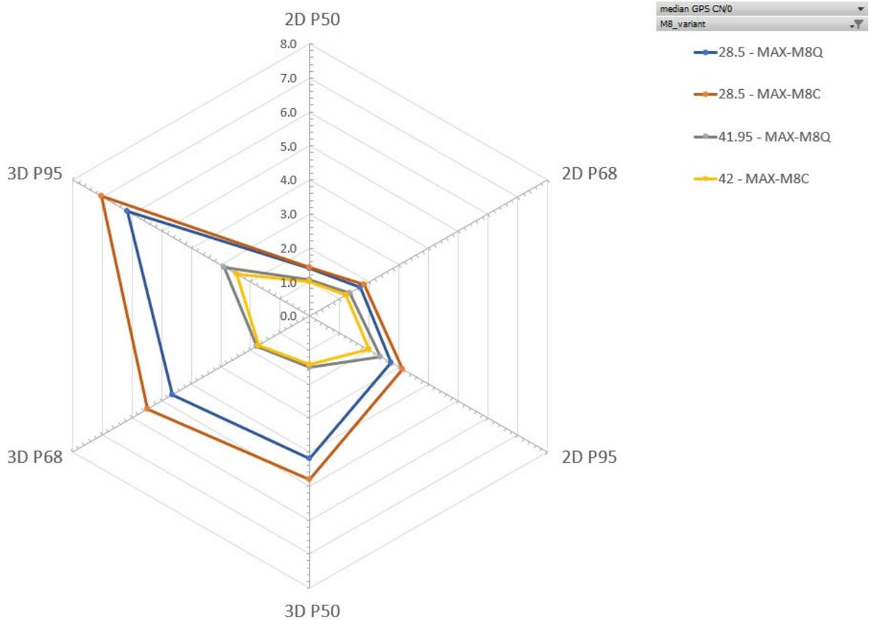
**Figure 9: Position error in meters for MAX-M8C and MAX-M8Q in percentiles at 28.5 and 42 dBHz in a highway test (default mode: GPS and GLONASS including QZSS, SBAS)**
