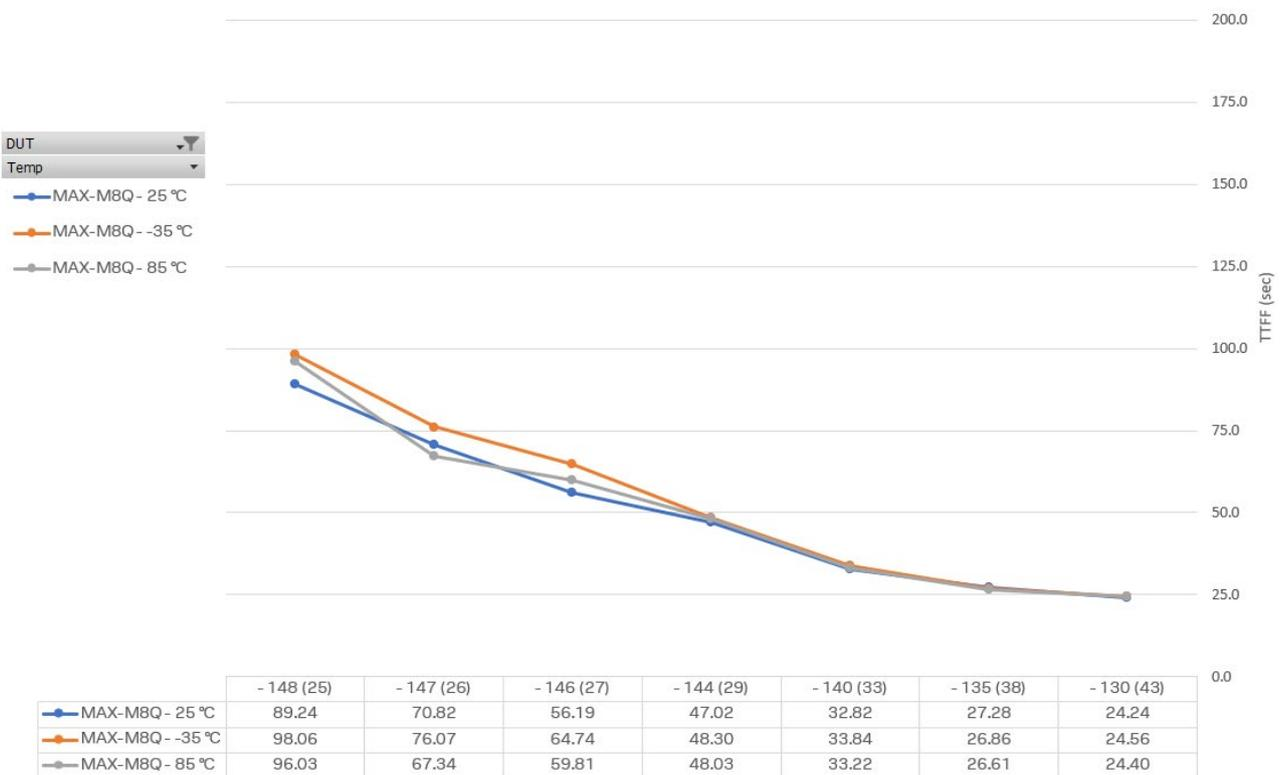
**Figure 4: TTFF vs. signal power in dBm and equivalent C/N0 inside parenthesis for MAX-M8Q during cold starts at +25, -35, and +85 °C (default mode: GPS & GLONASS including QZSS, SBAS)**
