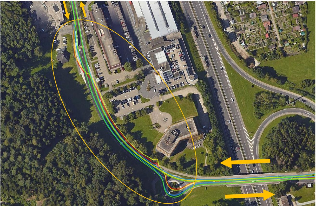
**Figure 14: Tracks for MAX-M8C (in blue), MAX-7Q (in yellow), and MAX-7C (in red), and reference position (in green) in an area with lower GNSS visibility**
