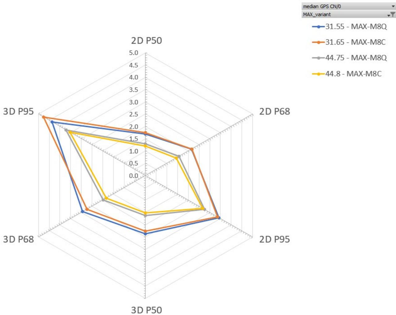
**Figure 5: Position error in meters for MAX-M8C and MAX-M8Q in percentiles at 31.6 and 44.7 dBHz in rural areas (default mode: GPS and GLONASS including QZSS, SBAS)**
