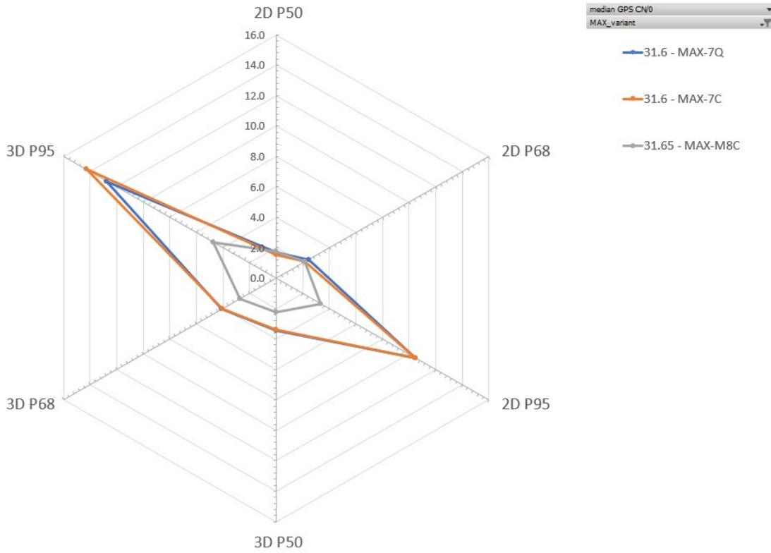
Figure 12: Position error in meters for MAX-M8C, MAX-7Q and MAX-7C in percentiles at 31.6 dBHz in a rural area
