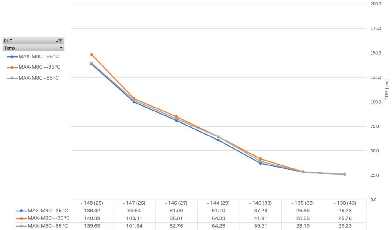
**Figure 3: TTFF vs. signal power in dBm and equivalent C/N0 inside parenthesis for MAX-M8C during cold starts at +25, -35, and +85 °C (default mode: GPS & GLONASS including QZSS, SBAS)**
