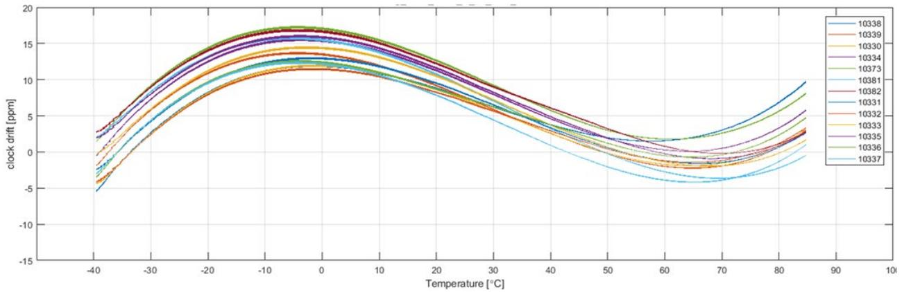
Figure 1: Temperature effect crystal on various crystal-based modules
