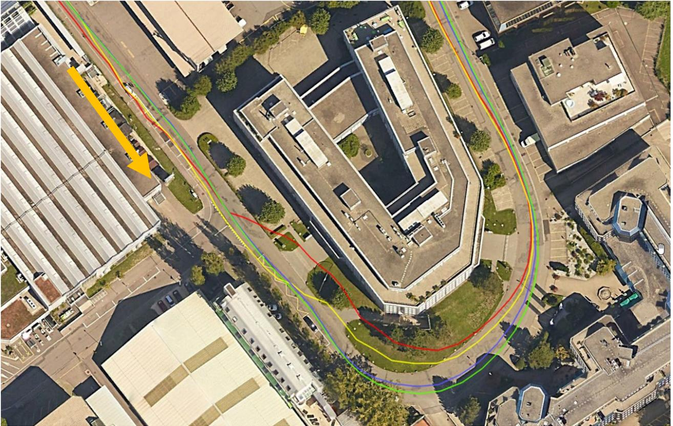
Figure 15: Tracks for MAX-M8C (in blue), MAX-7Q (in yellow), and MAX-7C (in red), and reference position (in green) in a narrow street
