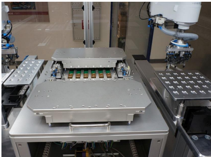
Figure 15: Automatic test equipment for module test
