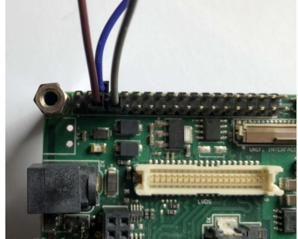
Figure 6: I2C interface on the TK1
