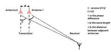
Using phase differences to derive the angle of departure. Adapted from Bluetooth SIG
