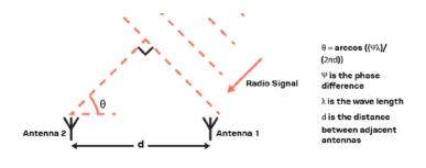
Using phase differences to derive the angle of arrival. Adapted from Bluetooth SIG
