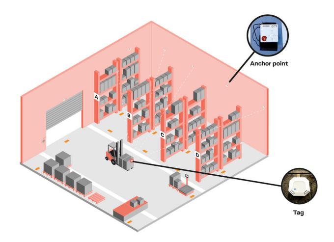
A typical setup to triangulate the precise location of mobile devices or tags in indoor environments comprises several multi-antenna anchors, as illustrated in the image below.
