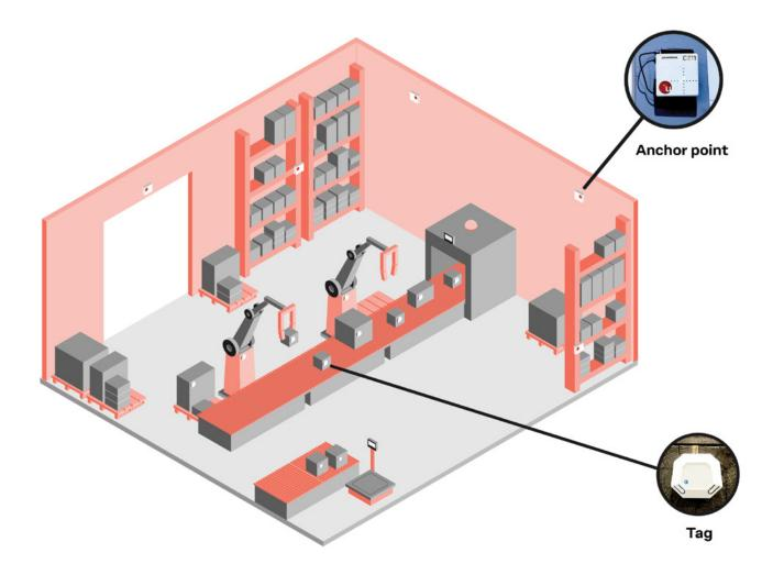
Illustration of an indoor positioning deployment in a production line.
