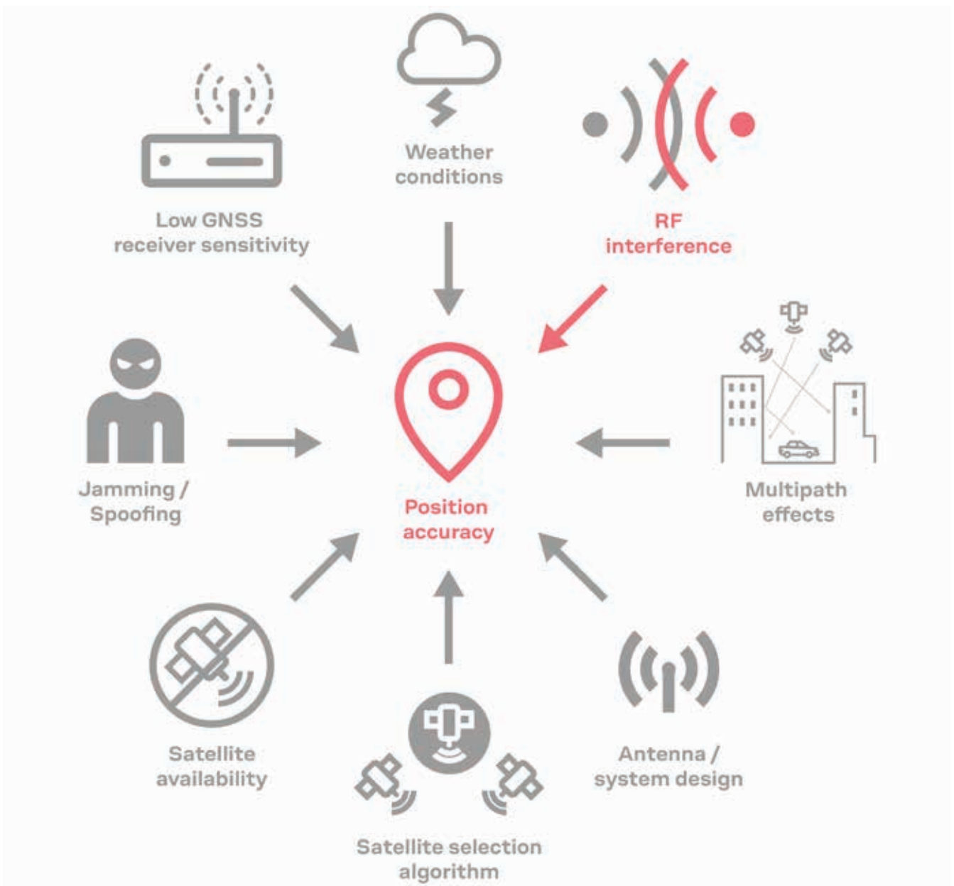
Image 2: RF interference is one of many factors impacting the performance of GNSS receivers.
