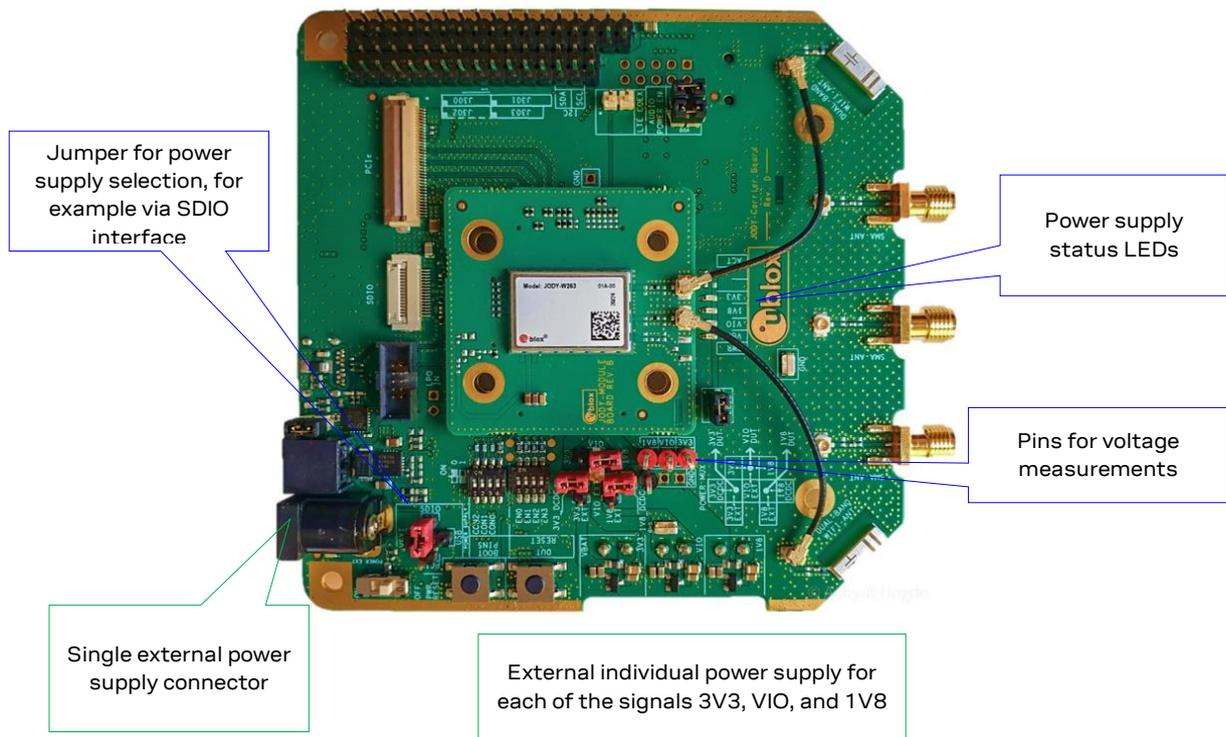
**Figure 9: Overview of EVB power supply configuration**
