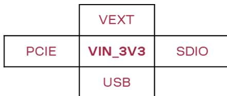
Figure 11: External power supply selection, J104-J106
