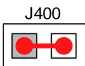
Figure 15: Jumper setting to use Bluetooth over USB
