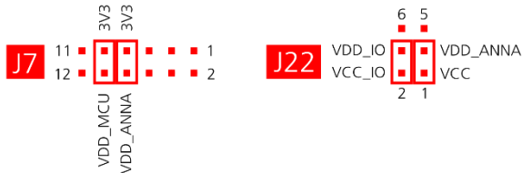
Figure 8: Jumper positions for default power configuration
