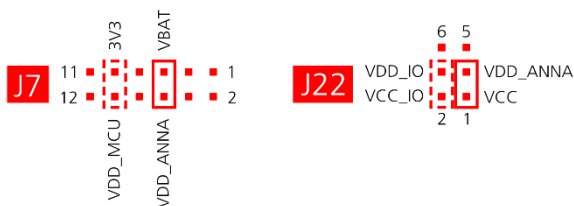
Figure 9: Jumper positions for battery powered operation, two jumpers are optional
